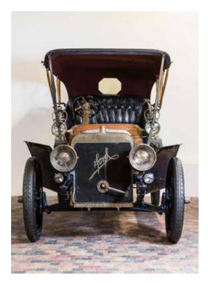
Carlton Pate has kindly provided the specific information that he has on this car, stating that it is an example of the early pattern 4-inch deep frame model, and is fitted with Kristoffy transmission, Stromberg glass bowl carburetor, aluminium blade fan and two coil boxes, all signifying its 1906 year. Other detail features which draw the eye are its tiny diagonal Ford script across the radiator, and the large Gray & Davis headlamps as well as their matched sides on the dashboard.
